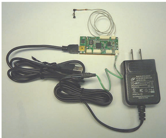
ST35B-14 Evaluation Kit connection
