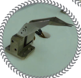
Minute clamp of the lens
