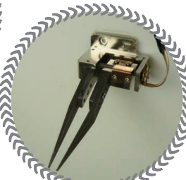
Soft body pickup clamp
